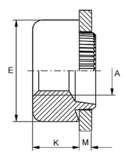
Female thread A = M3Height K = 3.0Outer diameter E = 8.0Plate thickness = 4.4 to 4.6
